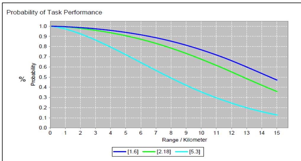
**Figure 8. Probability of detection of a human on land by distance using U.S. military modeling based on three levels of detection (from lowest to highest resolution): blue = detection, green = recognition, turquoise = identification (see Appendix A Glossary of terminology for evaluation of infrared/thermal technology as applied in this paper for definitions). (Source: NVTS 2020).**
